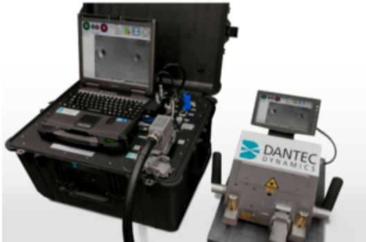
Q-810 Vacuum Hood Shearography [image source]
